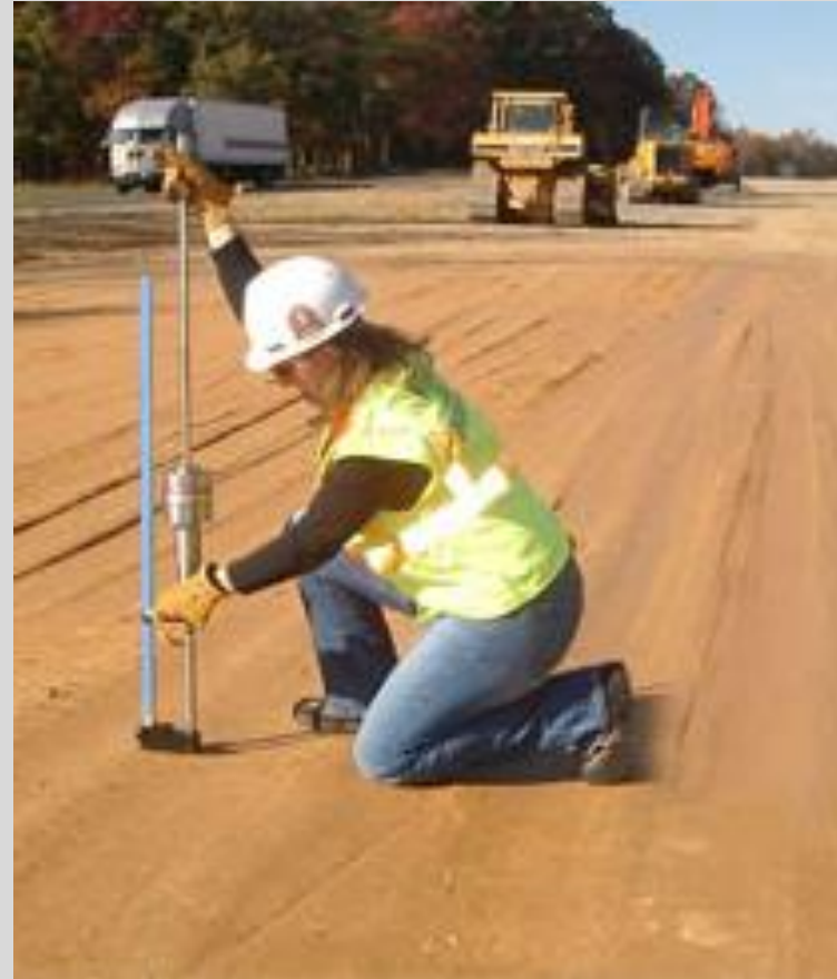
Field test - DCP
