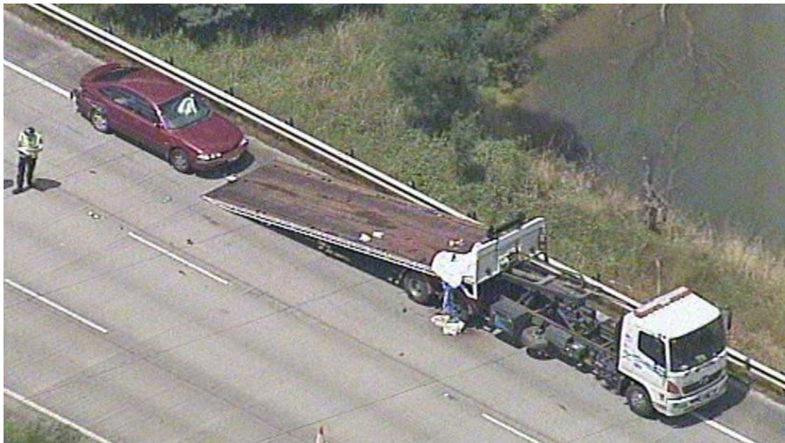
Figure 232: Vehicle not fully contained within shoulder
