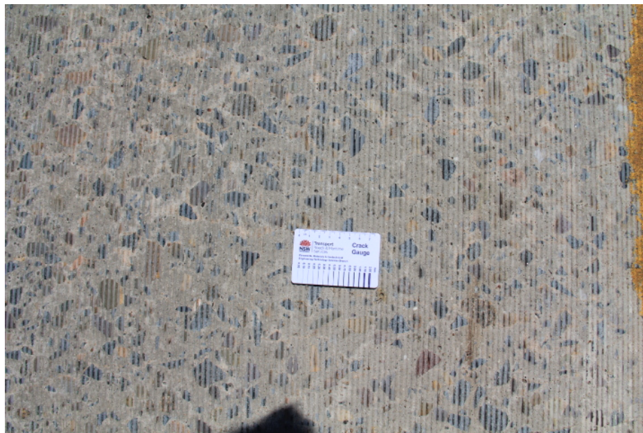
Figure 10. Surface of diamond grinding surface with the blade spacing set at 0.1 inches.
