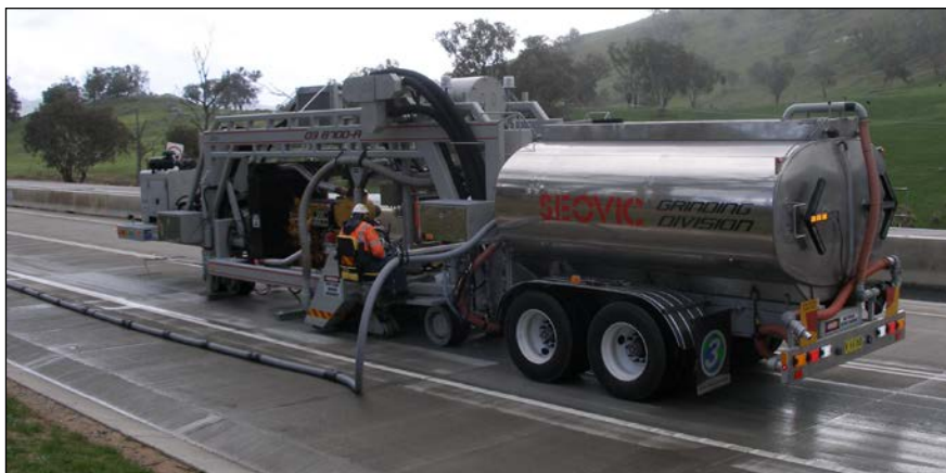
Figure 1. View of a diamond grind machine with a nominal 1.2 m wide grinding drum used on road pavements in Australia.
