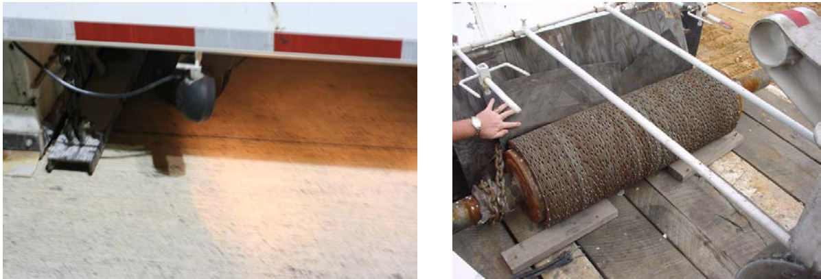
Figure 2. View of a magnetic collector in front of the grinding drum (left), and grinding drum showing numerous blades (right).
